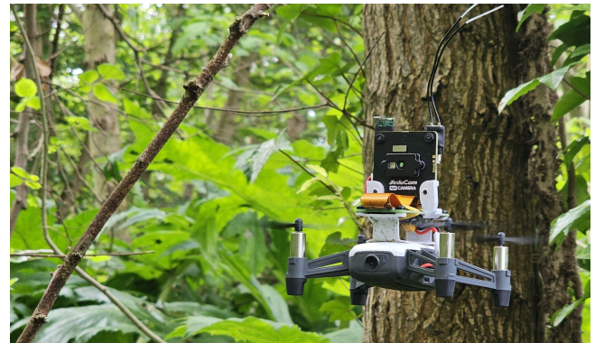
Figure 1: The 100-gram autonomous drone (DJI Tello with Raspberry Pi Zero 2W, and Arducam ToF camera) navigating in a dense forest.
