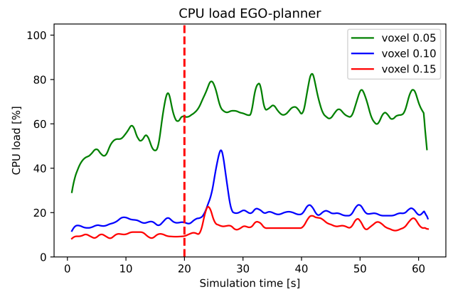
Figure 7: CPU load distribution over the benchmark simulation with voxel-grid resolutions of 0.05, 0.10, and 0.15 m.
