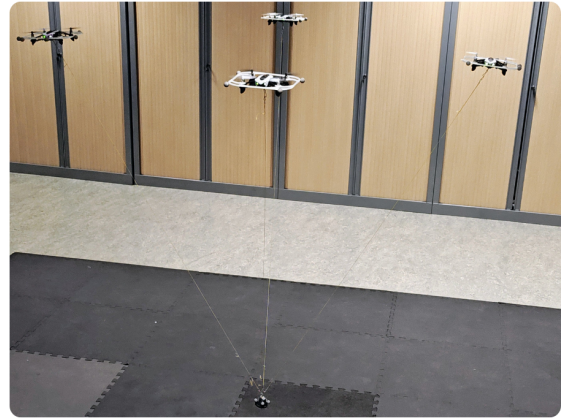
Figure 1: Experimental setup: four Parrot MAMBO mini-UAVs cooperatively carrying a cable-suspended load. A video of the experiments is available at youtu.be/fomDca2OPEA .
