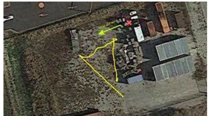
(b) GPS drone trajectory during the fire training container test (the drone trajectory is marked in yellow, the green arrow indicates wind direction, and the red cross marks the fire source).
