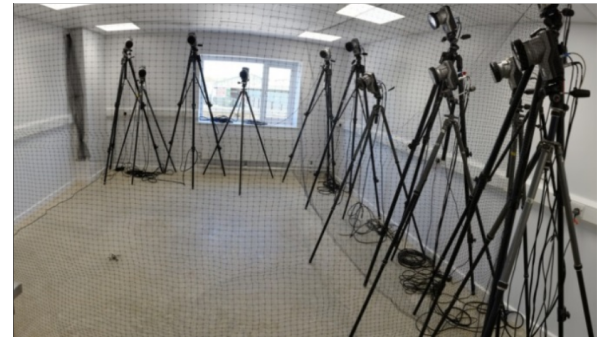
Figure 3: Image of the autonomous flight arena during its early development showing Qualisys motion tracking cameras and a Crazyflie UAV on the floor in the centre of a netted enclosure. This was used to track and control the Crazyflie during sense-and-avoid flight trials.
