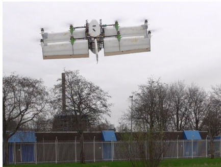
(a) Joint hover; Biplane in attitude INDI and quadrotor constant 70% thrust.
