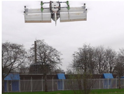
(b) Release mechanism engaged; The quadrotor has no attitude control.
