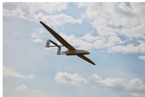
Figure 1: ELCOD Drone Stork Prototype - 5 m wingspan; 16 kg without payload; MTOW: 25 kg
