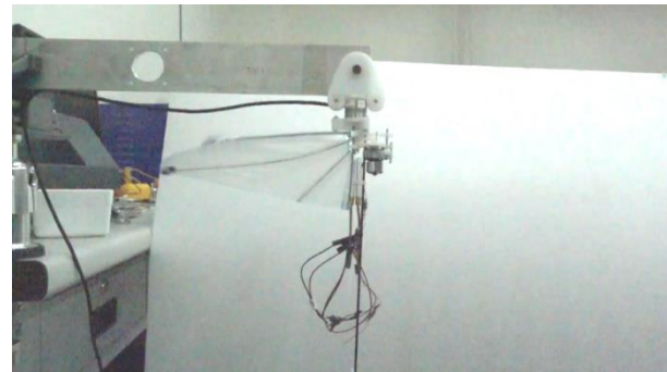
Figure 8: Equipment in force sensor thrust test.
