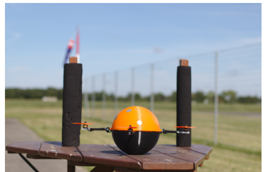
Figure 2: Quadrotor with custom spherical body shape
