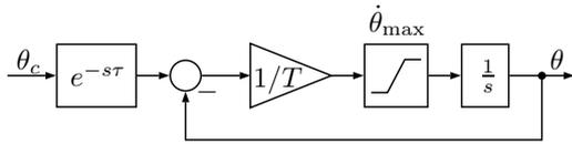
Figure 7: Actuator Model
