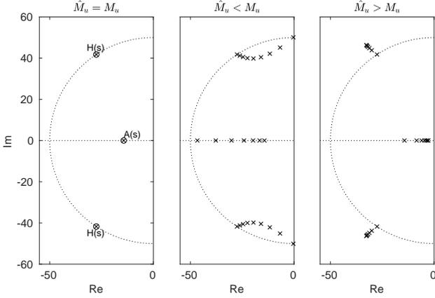
Figure 2: Effect of uncertainty in control effectivity on significant poles of INDI loop,  $0.2 < \hat{M}_u/M_u < 4$
