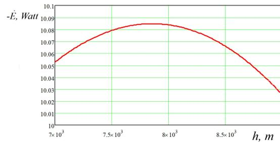
Figure 8: Accumulator incoming power as function of altitude near the maximum.
