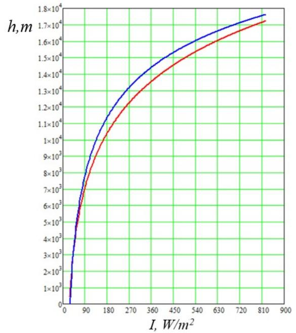
Figure 7: Altitude as function of solar intensity. Blue line — low atmosphere model (9), red line — isothermal model (10).
