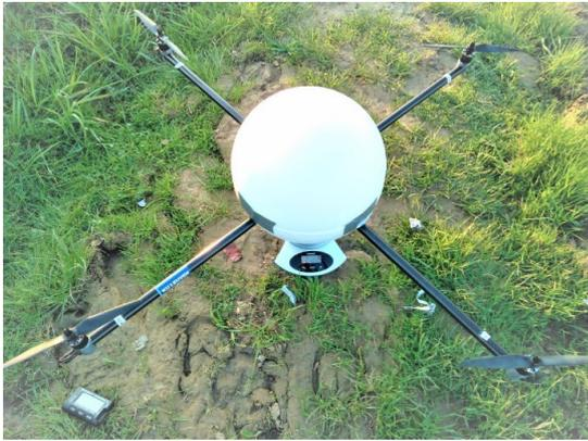
Fig. 3: Multicopter fitted with a  $40\text{cm}$  spherical *Styrofoam* body during mass check right before takeoff.
