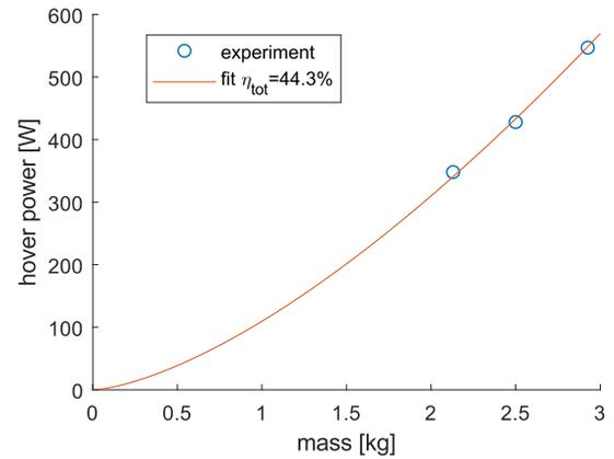
Fig. 13: Hover power and fit based on momentum theory with the assumption of a constant efficiency from battery power to kinetic energy of the accelerated air.
