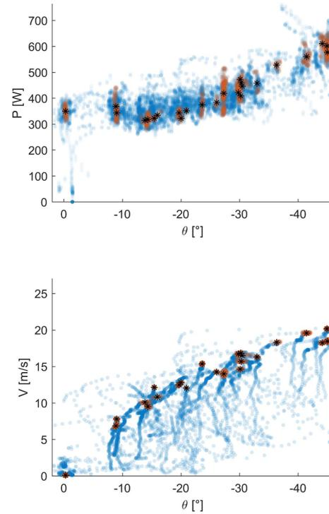
Fig. 5: Total power consumption and horizontal velocity as a function of the pitch angle for the configuration with  $2.13kg$  and  $40cm$ . Blue: all recorded data during the test flight. Orange: recorded data during identified steady-state regime. Black: average values for each steady-state regime
