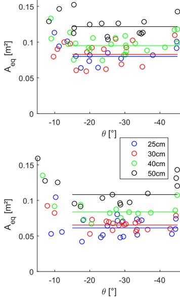
Fig. 11: Calculated equivalent frontal surface at pitch angles from hover to  $-45^\circ$  for four different body diameters and two total masses. The horizontal lines present the mean value for pitch angles from  $-15^\circ$  to  $-45^\circ$ .
