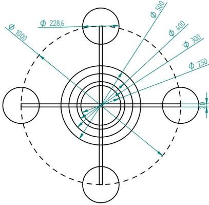
Fig. 2: quadcopter dimensions in  $\text{mm}$  with four different possible diameters of spherical body.
