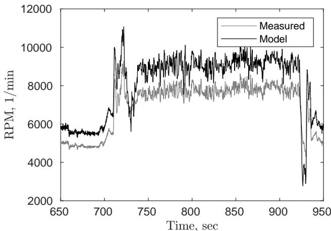
Figure 8: BLDC/ESC model
