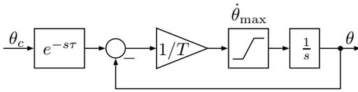
Figure 7: Actuator Model
