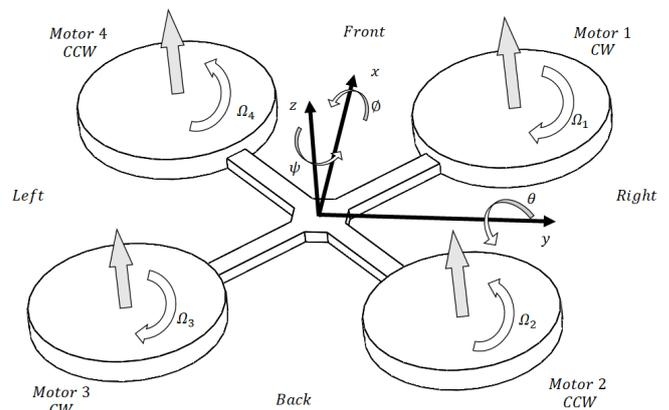
Figure 1: Quadcopter Representation
