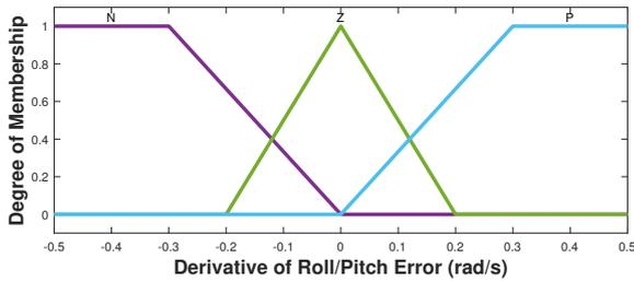
Figure 12: Input Membership Function - Derivative of Roll/Pitch Error
