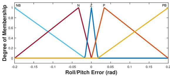
Figure 11: Input Membership Function - Roll/Pitch Error
