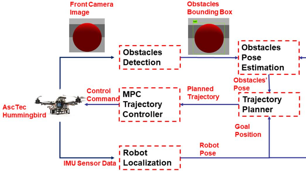
Figure 2: Architecture of the autonomous navigation method proposed.
