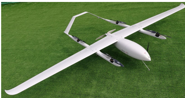
Figure 2: Eagle Plus VTOL UAS. Source: Sparkle Tech [3].
