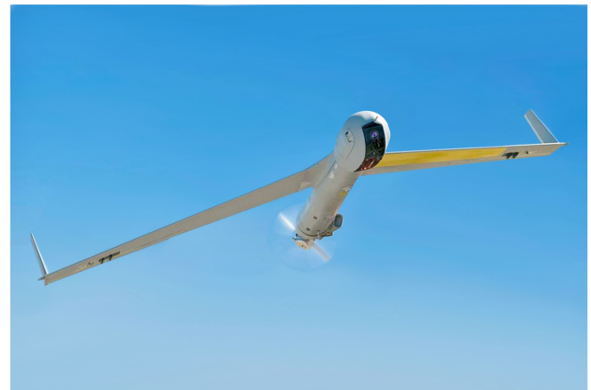
Figure 5: Scan Eagle UAS. Source: Insitu [7].
