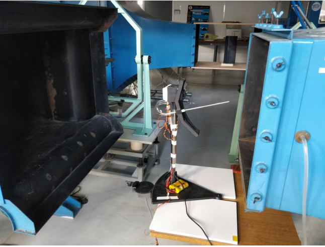
Figure 12: Calibration bench located inside the test section of ENAC's low speed wind-tunnel.
