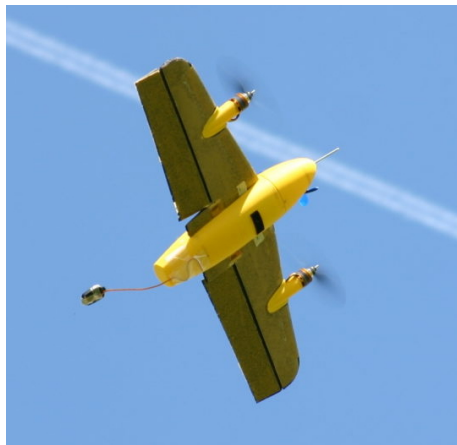
Figure 2: Convertible UAV Cyclone hovering with negative flap deflection
