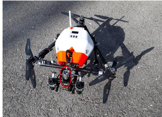
Figure 1: Multicopter “ARDEA” with a frame in triangle shape, three pairs of counter-rotating rotors and a sensor suite mainly consisting of an IMU, two pairs of wide-angle stereo cameras and an insect-inspired polarization compass (highlighted by red ellipse).
