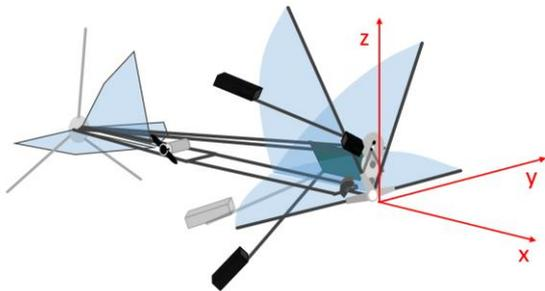
Figure 4 - Definition of internal axes of WiFly
