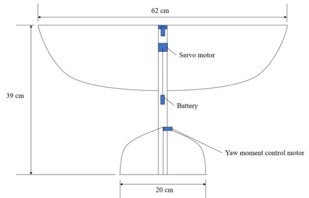
**Figure 2 – Dimensional outline of WiFly and components arrangement**
