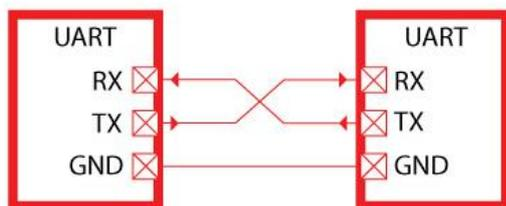
Figure 3 – Connection between Devices Using UART Ports
