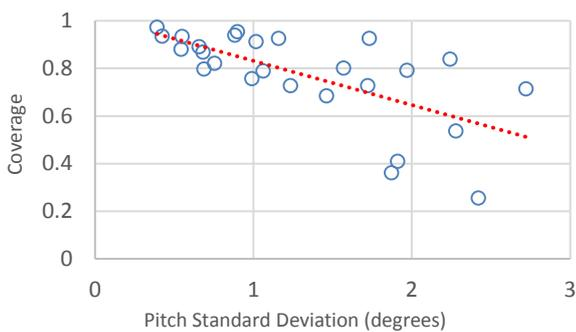
**Figure 8 – Coverage vs UAV pitch variation**
