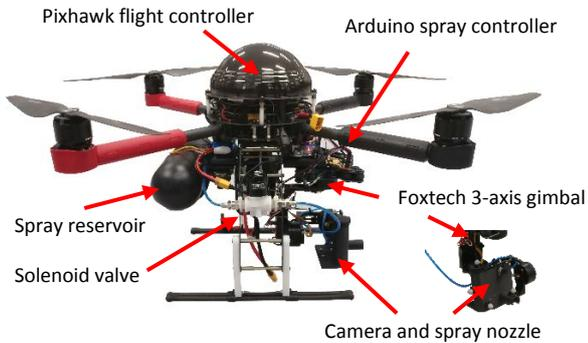
**Figure 1 - Multirotor UAV with spray system**
