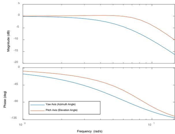
Figure 4 - Bode plot for gimbal yaw and pitch
