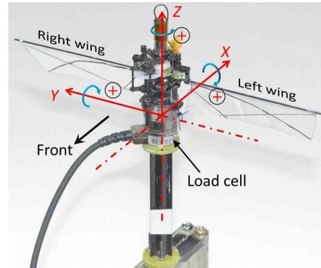
**Figure 3 – Experimental setup for forces and torques measurement using a load cell**
