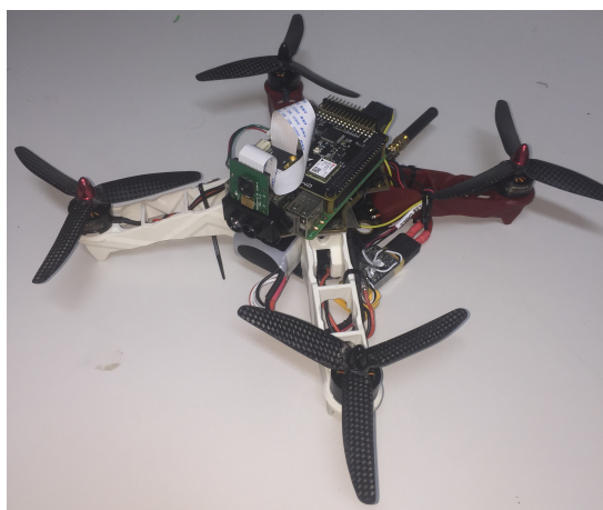
Figure 2: MAV used during the tests with LiDAR sensor mounted.
