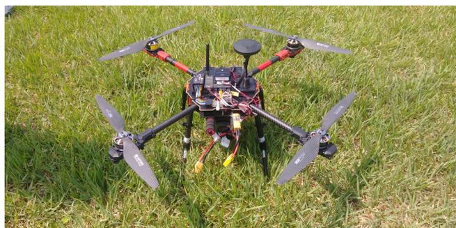
Figure 14: UASG-DOBC-Quadrotor.
