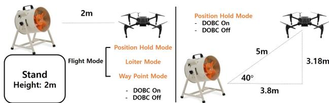
Figure 17: Flight test method using blower fan.
