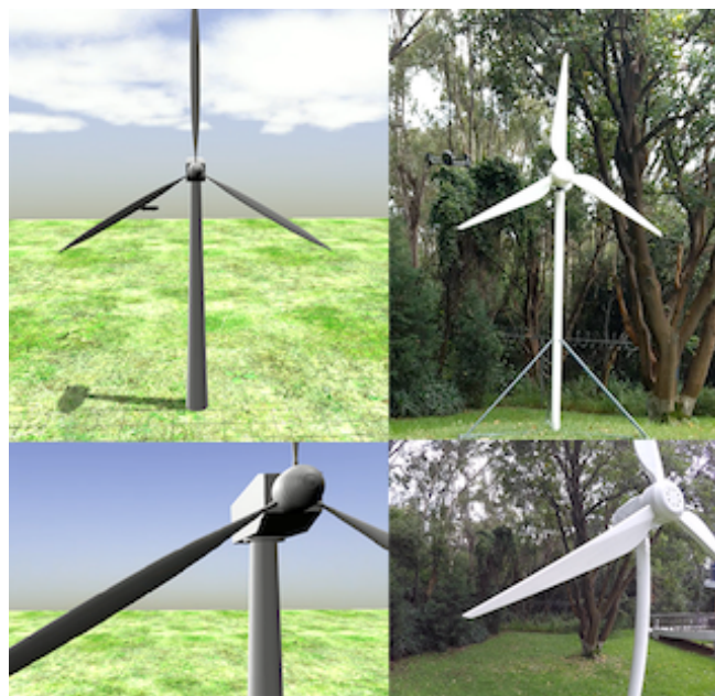
Figure 1: Left column: simulated inspection using Gazebo, with the bottom image showing the view of the frontal camera; right column: likewise, inspection carried out on an emulated turbine. https://youtu.be/XZZm345rCRY
