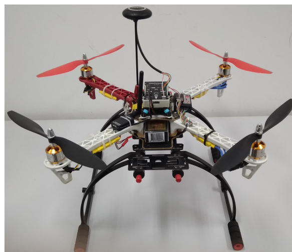
Figure 2: Developed UAV quadrotor
