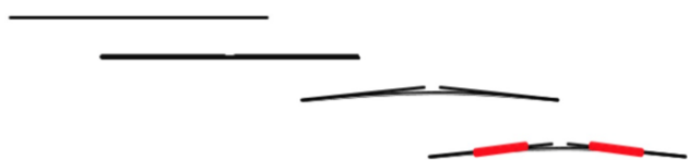
Figure 3: Process of delamination of the carbon fiber rods.
