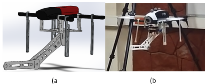
Figure 3: Aerial Manipulation system implemented for this work.
