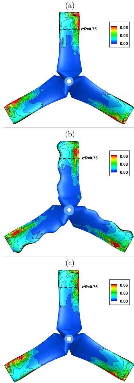
Figure 5: Time-averaged solution on the suction side colored by the normalized pressure fluctuations  $p' / (\frac{1}{2}\rho(\Omega.R)^2)$ : (a) reference geometry, (b) wavy leading edge and (c) shifted blades.
