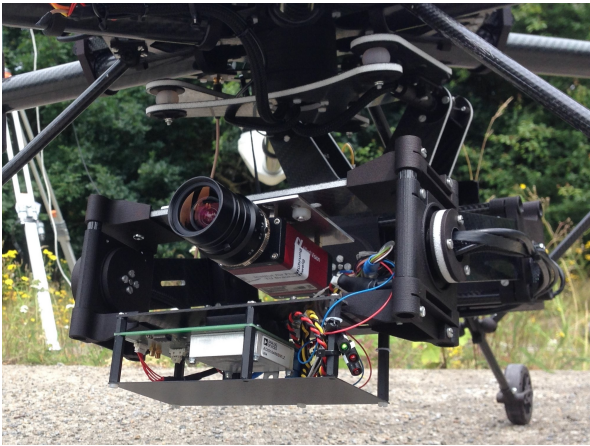
Figure 2: Gimbal with Camera and IMU.
