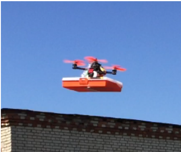
Figure 1: Copter of first design in flight with cargo fixed "horizontally"
