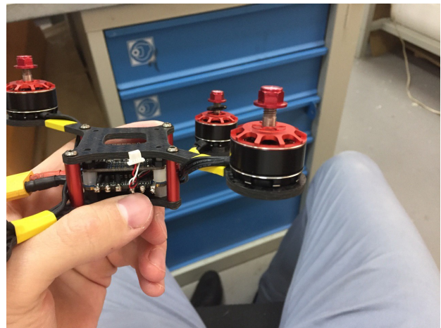
Figure 3: Double deck frame
