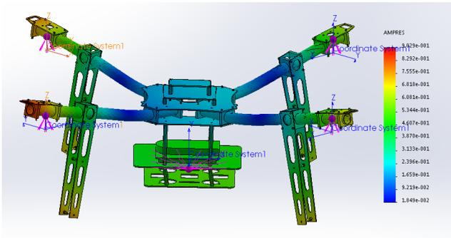
Figure 3: Mode shape of T-Lion at 109.88 Hz
