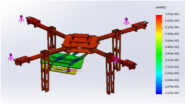
Figure 2: Mode shape of T-Lion at 39.9 Hz
