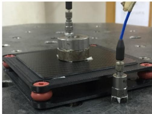
Figure 6: Vibration test setup on vibration table
