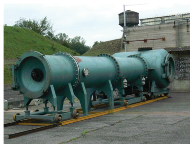
(b) 18 m 3 depressurized tank located at ONERA's Fauga center
