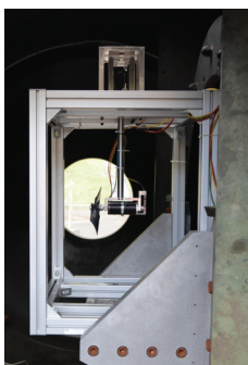
(a) ISAE-SUPAERO's experimental testbed in the depressurized tank
