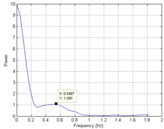
Figure 4: Sample 2 of dutch roll mode frequency.
