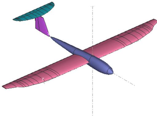
Figure 6: Sonic 185 including fuselage in XFLR5.
