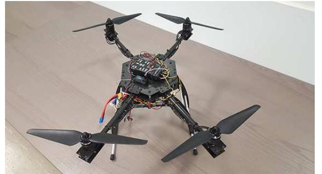
Figure 9: Assembled quad-copter configuration
