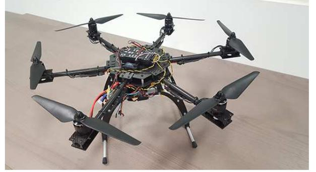
Figure 8: Assembled hexa-copter configuration
