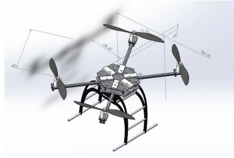
Figure 5: SolidWorks impression of quad-copter configuration
