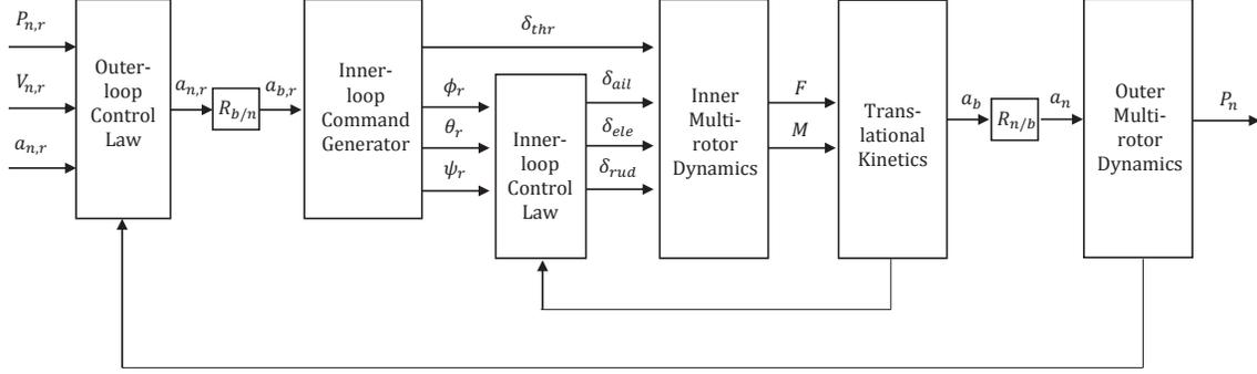
Figure 7: Flight control block diagram
