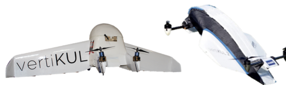
Figure 1: Left: VertiKUL 1, designed to make a transition of 90^\circ with a large wing to provide all the lift. Right: VertiKUL 2, designed to make a transition of 45^\circ with smaller wings to improve wind gust resistance.
