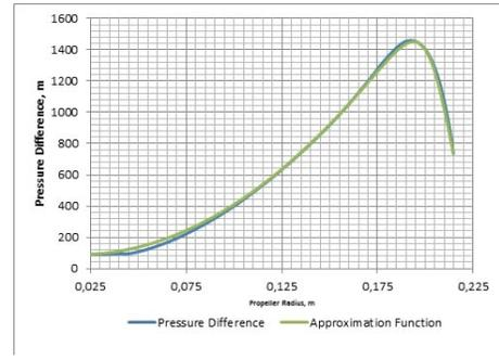
Figure 2: Pressure difference between upper and lower surfaces of the propeller on its quarter chord line.
