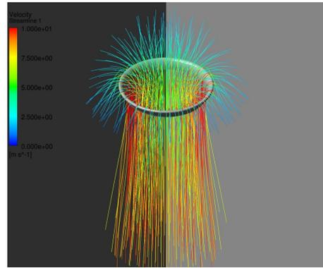
Figure 9: Streamlines that passes the actuator disc.
