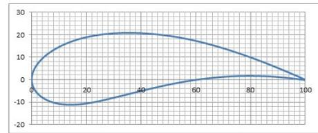
Figure 3: Airfoil obtained from the optimization task.
