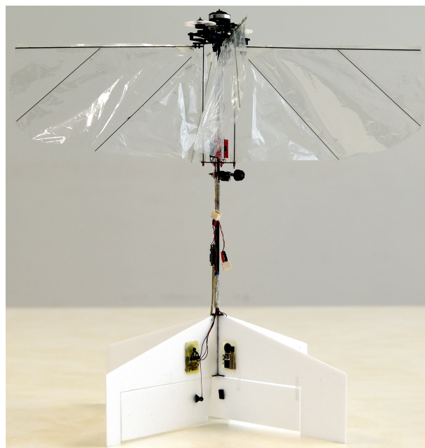
Figure 1: The FlowerFly with onboard camera and control system for pitch-, yaw-, and roll-control controlled by three servos.
