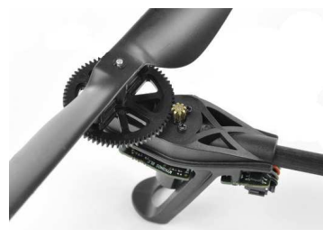
Figure 2: The motor's and the propeller's gear wheels.
