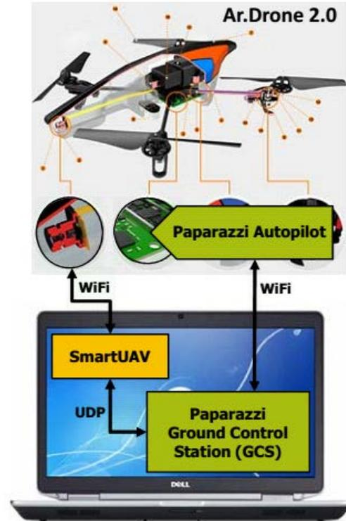
Figure 1. Test bed system architecture [38]
