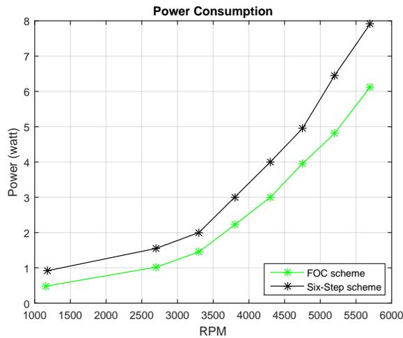
Figure 9: Power consumed by the motor under different speed for rotor combo of hexTronik outrunner 1700 kV and 6030 propeller.
