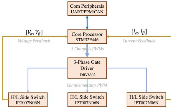
Figure 5: FOC hardware development: function blocks incorporated.
