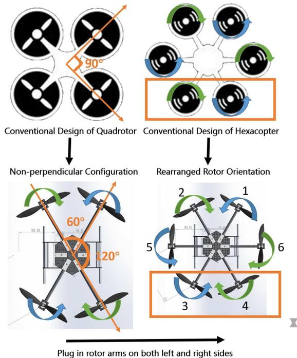
Figure 4: Graphical illustration of hardware modifications
