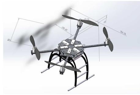
Figure 5: SolidWorks impression of quad-copter configuration
