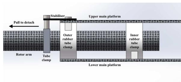
Figure 3: SolidWorks impression of the connection mechanism
