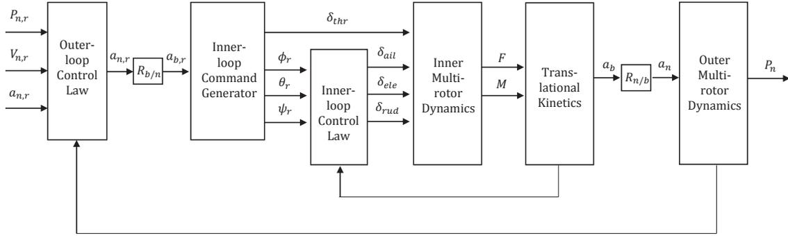
Figure 7: Flight control block diagram
