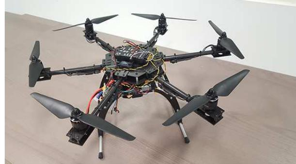
Figure 8: Assembled hexa-copter configuration
