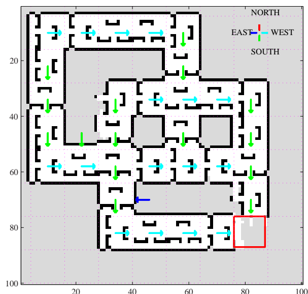
Figure 5: The greedy macro actions in the memorized map after 15 iterations with hierarchical Q-learning.
