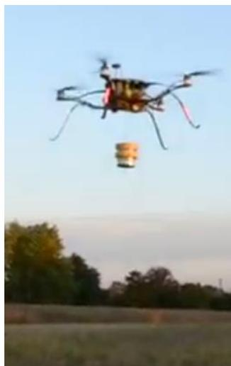
Figure 11: Bambi-Bucket attached to the MAV
