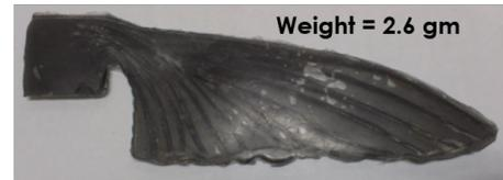
Figure 11: Bio-mimicked hummingbird wing.
