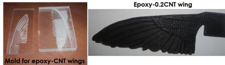
Figure 10: Epoxy-CNT composite wings.
