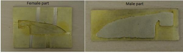
Figure 4: Manufactured Lower and Upper Mold for PP Wing.
