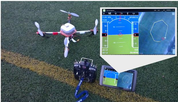
Figure 16: Android-based Ground Control Station
