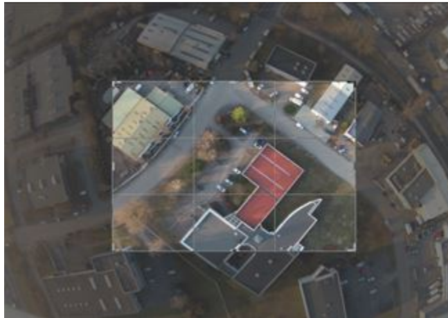
Figure 2: crop made around the non-distorted zone, image taken during a flight test
