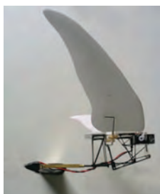
Figure 1: Flapping-wing MAV mounted on the force balance
