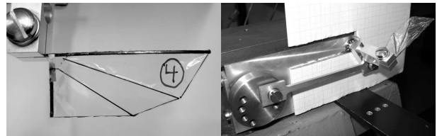
Figure 6: The completed wing showing the wing hinge structure (left) and the wing test setup (right)
