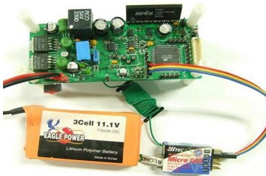
Figure 7: The implemented hardware of MIPAD (100mm x 40mm, 53.3g).
